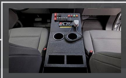
**POLYUREA SPRAYED ALL ALUMINUM FRONT CONSOLE - INTERCHANGEABLE DESIGNS**
